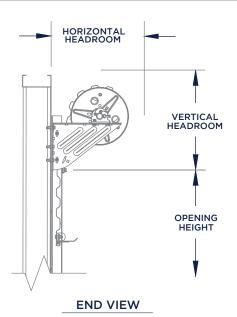
Universal mount 2.25" deep 16-gauge galvanized steel guides require no pre-installation modifications for wood, steel, concrete or filled masonry block applications.
